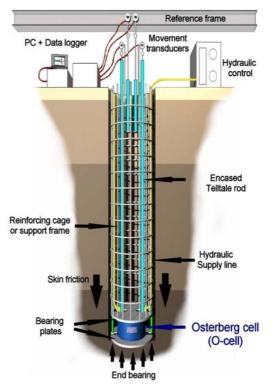
Figure 5.5 Schematic details of system
