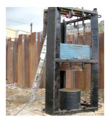
Figure 5.9 Dynamic load testing of cast-in-place pile
