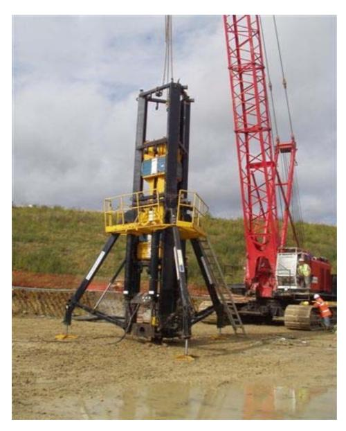
Figure 5.7 3MN capacity test
