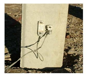
Figure 5.9 Strain gauge and accelerometer bolted to precast concrete pile The arrangement is repeated on the opposite pile shaft face
