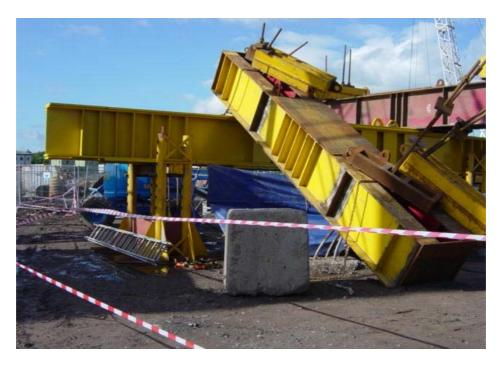
Figure 2.1 Failure of tension bar system in reaction pile
