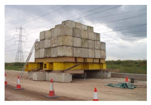
Figure 5.3 3MN kentledge test
