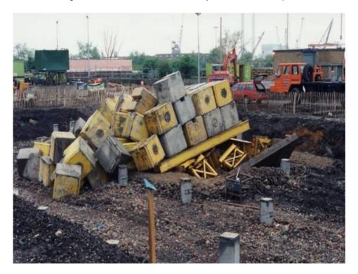
Figure 2.2 Platform bearing failure under kentledge test
